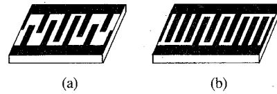
Fig. 10. Examples of (a) apodized IDT and (b) withdrawal weighted IDT to realize a resonator with three resonances described in Fig. 8(b).
